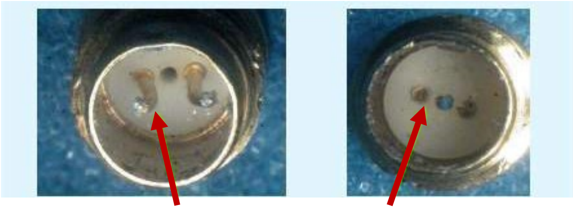
Bent or Broken Pins due to scooping or stubbing
